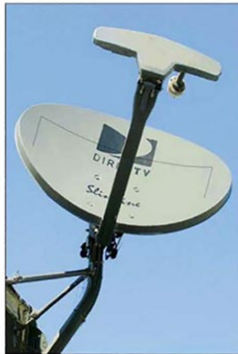
Figure 1 — Note the low visibility of the slot in my modified satellite TV dish.
